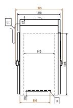
Drain Electrical inlet (power) ΕI Refrigerant Outlet
